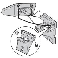
Adjust the adaptor to hold the base unit, then push it in the direction of the arrow until it clicks into place.
